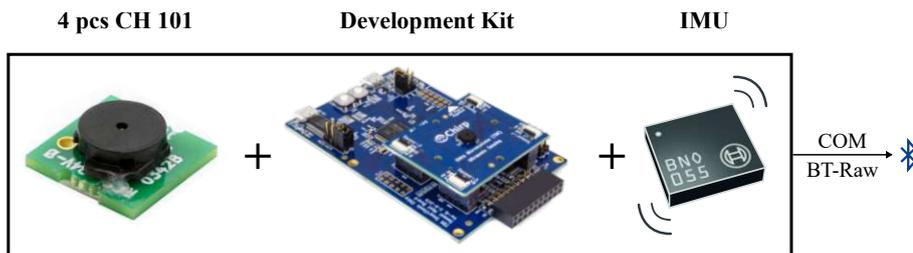
**Figure 2.13:** Block Diagram of the CoLiRang system kit. Ultrasonic sensors measure the distance to the sound-side leg, which is streamed to a laptop via a bluetooth module.
