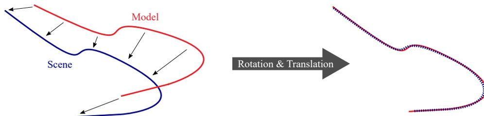
**Figure 2.6:** Principle of the iterative closest point method. The scene (blue) is kept fixed, while a model (red) is transformed (rotation and translation) to best match the input.
