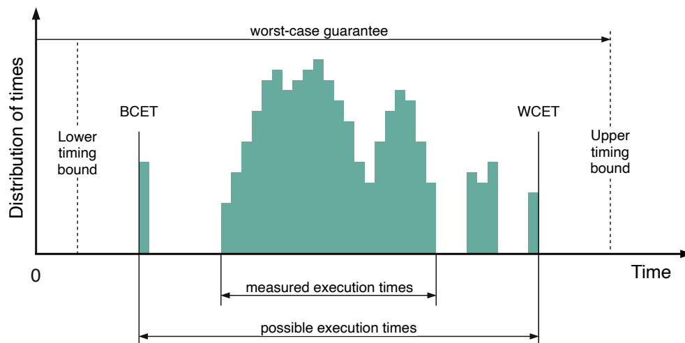
Figure 2.3: Basic notions of timing analysis (adapted from [9])
