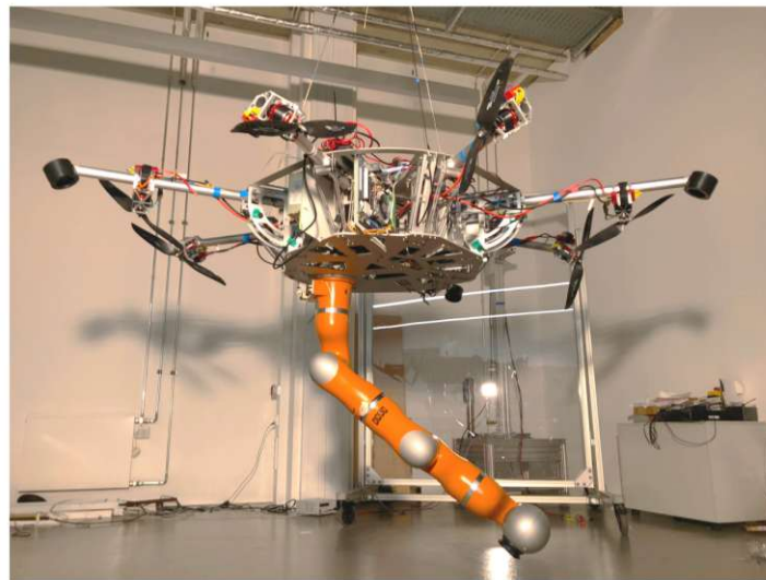
Figure 2.2: Prototype of Suspended Aerial Manipulator, reprinted from [6]
