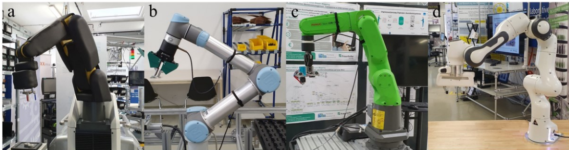
Figure 3 Photographs of different cobots used in the TU Wien Pilot Factory for Industry 4.0 in Vienna, Austria. (a) Bosch APAS, (b) Universal Robot UR5, (c) Fanuc CR-7iA, and (d) Franka Emika Panda (own figure).
