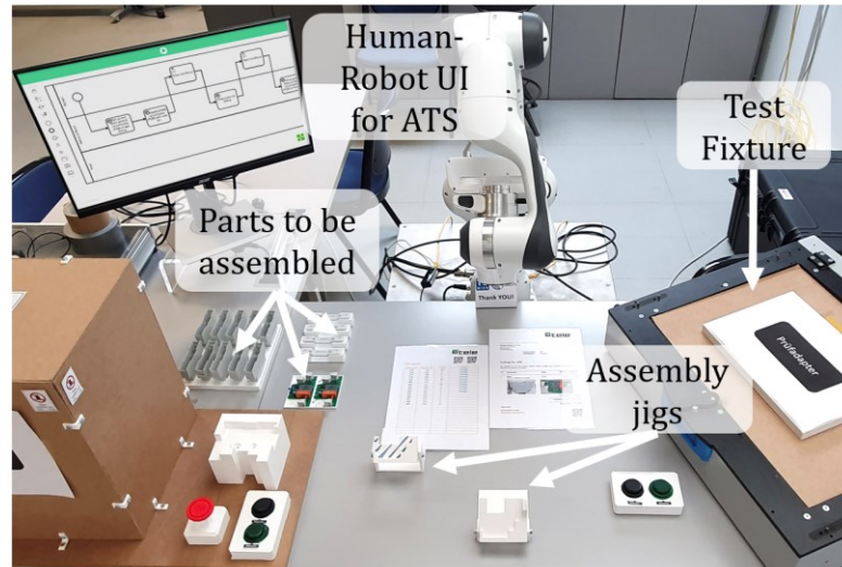
Figure 34 Use-case II “assembly of a timing relay” demonstrator at TELE Haase Steuergeräte Ges.m.b.H in Vienna, Austria (own figure).
