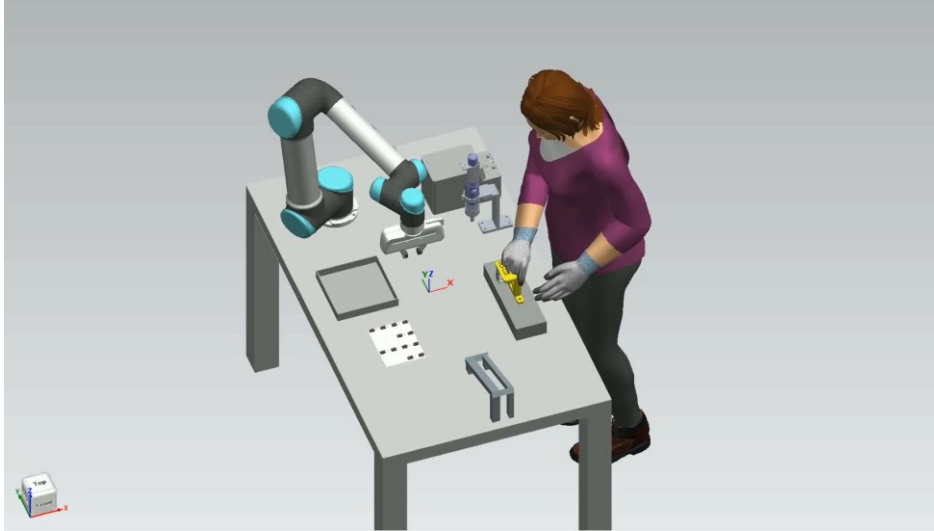
Figure 31 Virtual HRI workplace in Tecnomatix Process Simulate 15.0 (own figure).
