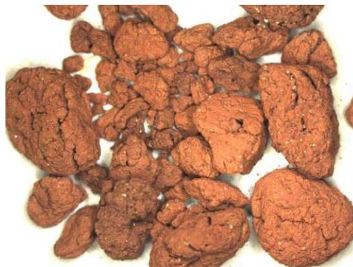
Figure 24: bottom ash experiment 1, inclusion of bed material particles
