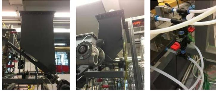
Figure 7: Bunkers and flushing system used during the experiments: small bunker (left), big bunker (middle), N<sub>2</sub> flush of bunkers (right)
