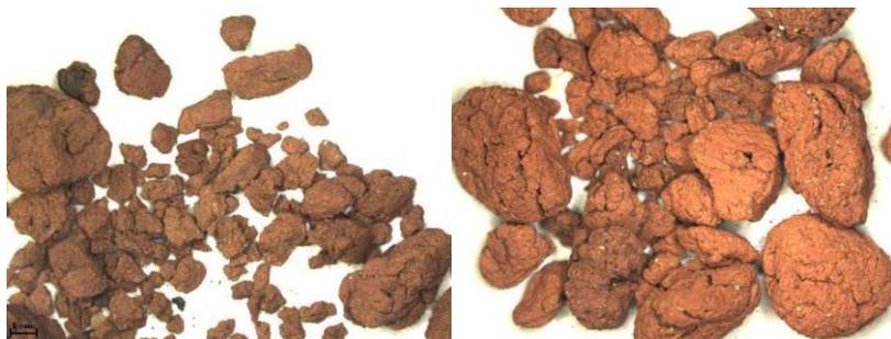
Figure 74: Light microscope image of the bottom ash in experiment 4 (left) and experiment 1 (right)
