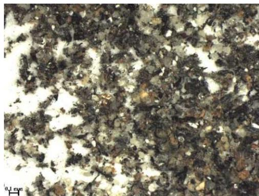
Figure 61: light microscope image cyclone ash, experiment 3
