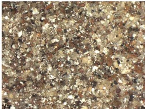
Figure 30: Light microscope image of cyclone ash, experiment 1
