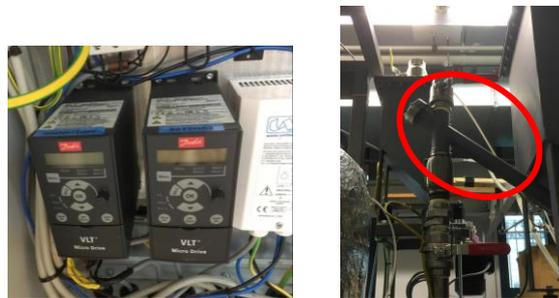
Figure 8: The feed flow is regulated by setting the rotation frequency of the screw conveyor (displayed on the left). The screw conveyor can be seen on the right.
