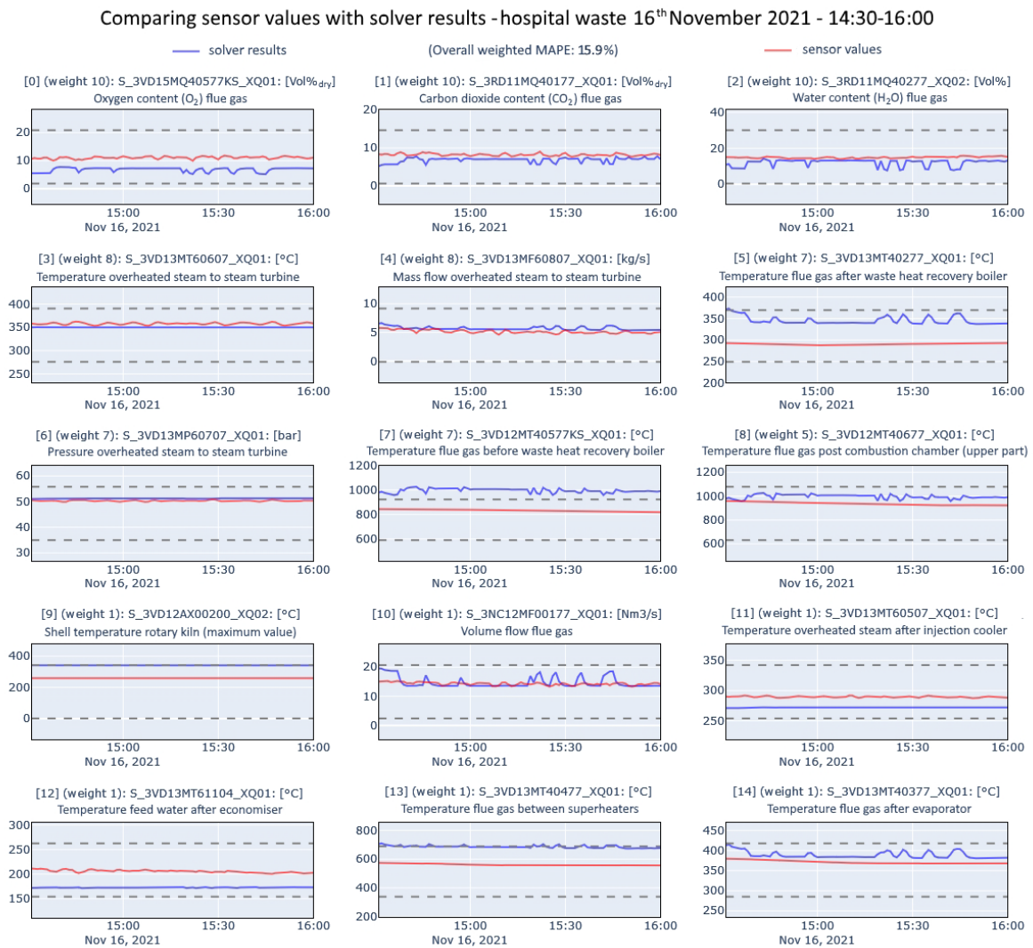
Fig. 33: Simulation and validation results for the exemplary determination of the waste composition for a not analysed hospital waste fraction [163]
