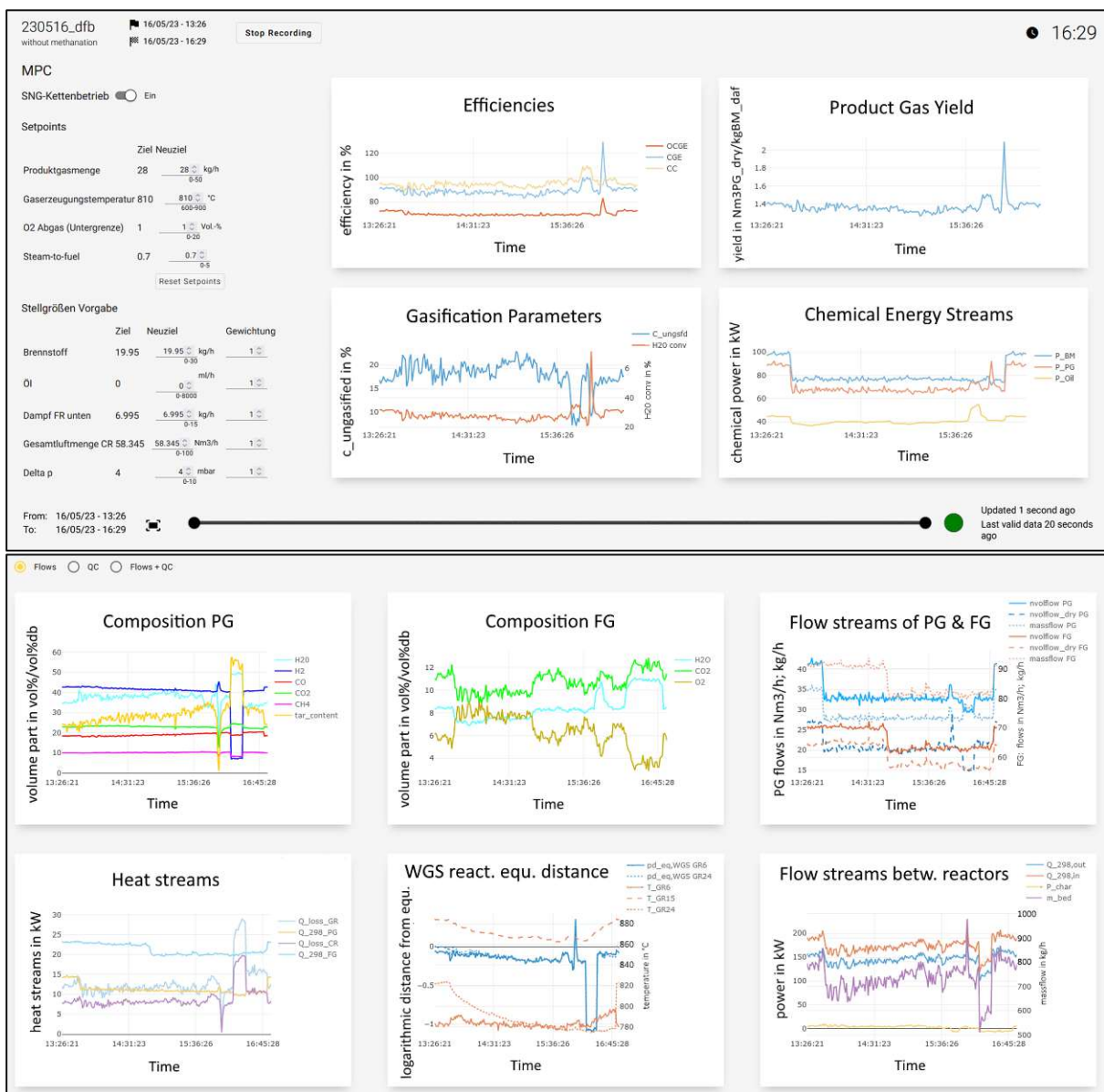
Fig. 29: Dashboard of the IPSEpro simulation results with the MPC human interface and the sustainability indicators (top) and results for important process parameters (bottom)
