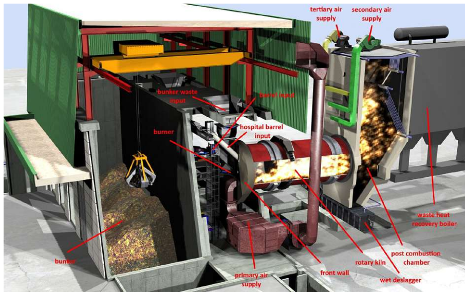
Fig. 2 3D visualization of the hazardous waste rotary kiln incinerator in Vienna at Simmeringer Haide [38]
