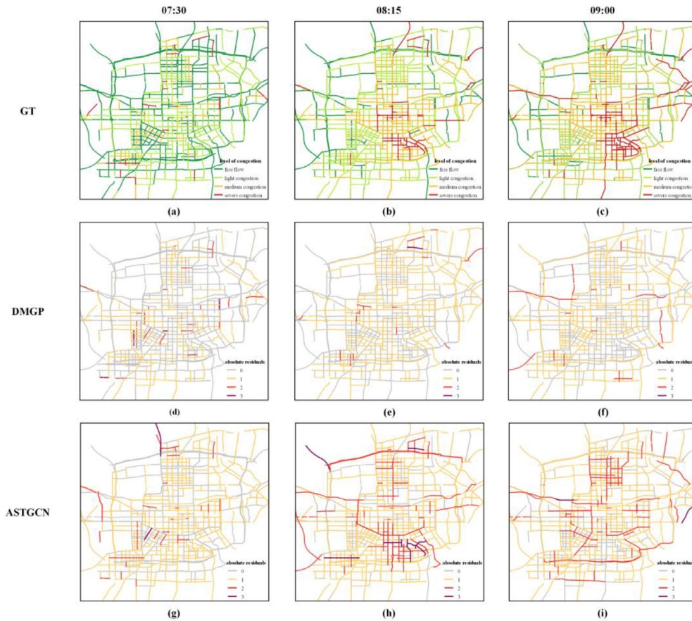
FIGURE 7 Examples of predicted congestion during the morning peak hour (7:30–9:00 a.m.) in Xi'an City. First row: ground truth; second and third rows: the difference between the congestion severity level predicted by deep marked graph process (DMGP)/attention-based spatial-temporal graph convolutional network (ASTGCN) and the ground truth.
