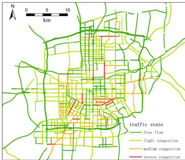
FIGURE 5 Road network in Xi'an City. Road segments are rendered in four colors to indicate different levels of congestion (severe congestion, medium congestion, light congestion, and free flow).
