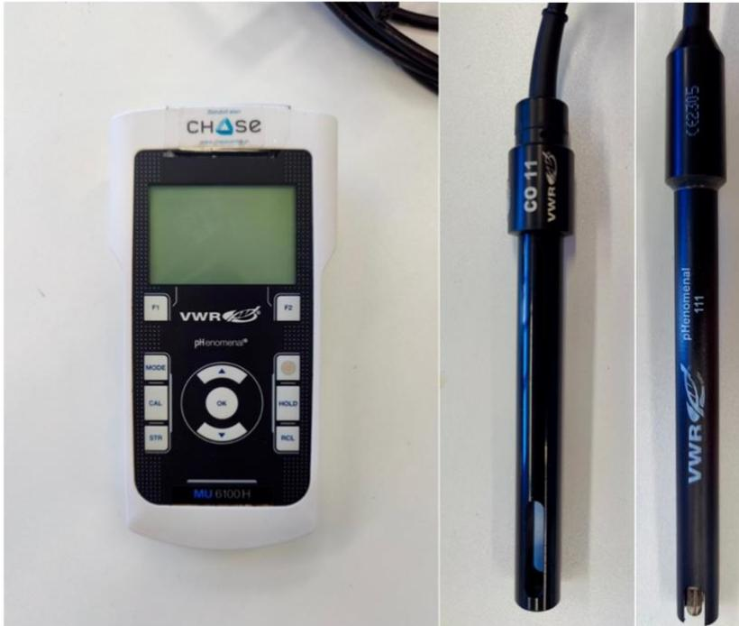
**Figure 13** MU 6100H Unit, Conductivity Sensor, pH Electrode
