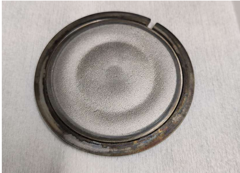
Figure 3: Metallic YSZ target with circular racetrack.
