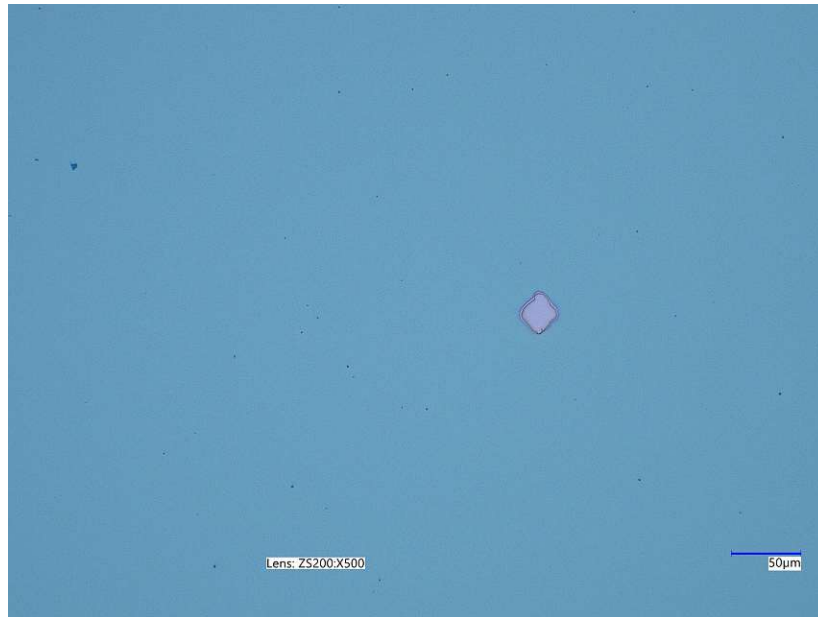
Figure 21: Cleaned YSZ surface with pinhole.
