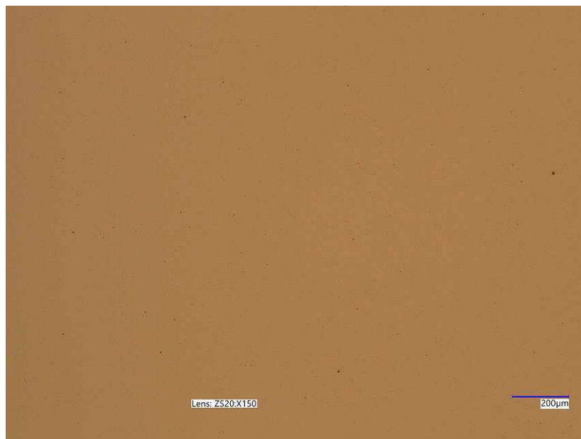
Figure 19: Cleaned Pt surface.
