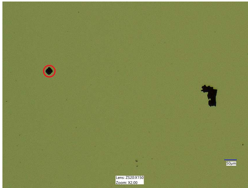
Figure 20: Sputtered YSZ layer uncleaned.
