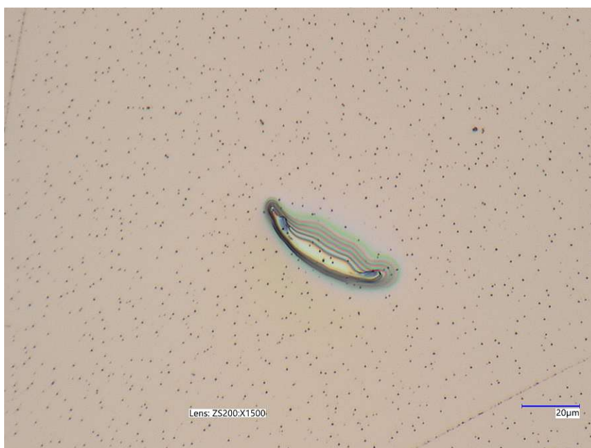
Figure 16: Pinhole due to a dirt particle of YSZ_25.
