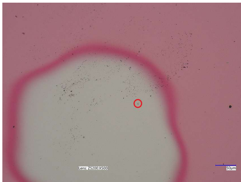
Figure 26: Microelectrode of YSZ 30 with a short circuit. The area with the possible pinhole is marked with a red circle.
