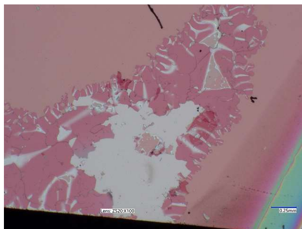
Figure 29: Detached thin film of YSZ_29.
