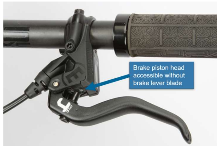
Figure 5.5: The Magura MT4 Model with the accessible brake piston head.
