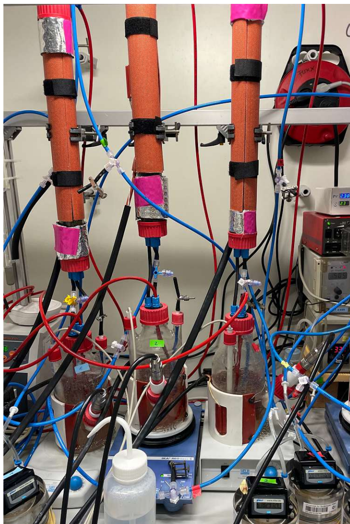
Figure 14: Trickle bed reactors - from left to the right: FR1, FR2 & FR3
