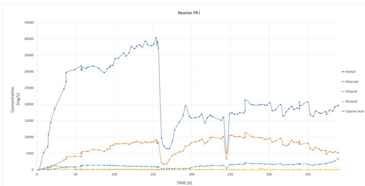
Figure 50: Concentration of acetate, butyrate, caproate, ethanol, butanol & hexanol in trickle bed reactor FR1 over time
