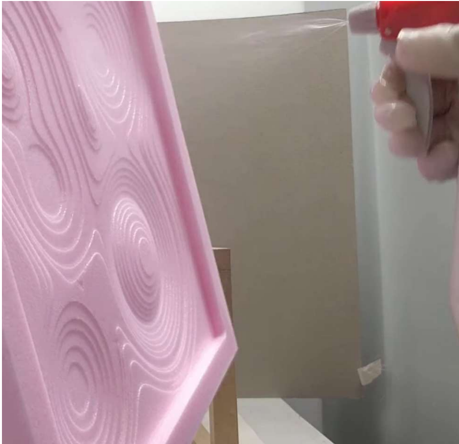
5.7 Vegetable oil as coating agent. The oil is applied by spraying.
