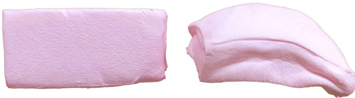
3.11 Comparison of 40 mm sample submerged for 10 min and 40 mm sample submerged for 6 h at 80%.
