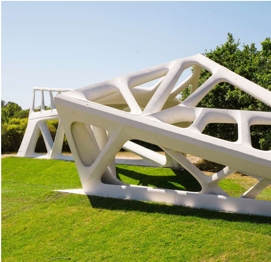
2.12 Prototype fabricated using abra- sive wire cutting by Søndergaard, et al. 2018
