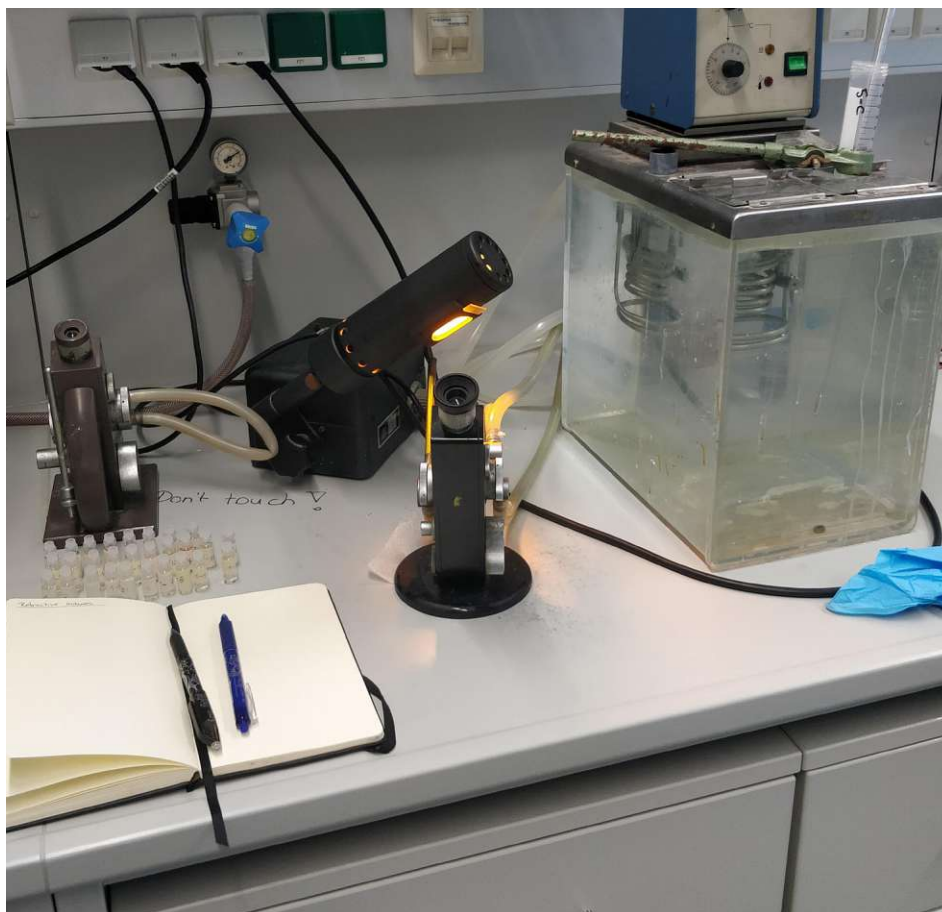
3.3 Workstation at the chemistry lab with the refractometer used for the measurements.
