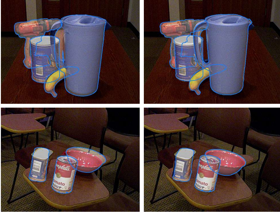
Figure 7.7: SporeAgent with Stable Pose Estimation on YCB-Video. Note that the stable poses (left) of the two cans in the bottom row are upside down. The refined poses (right) thus may achieve a low ADI error, while the ADD error remains high.
