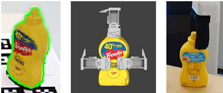
Figure 5.10: Refined estimates using RIR (left), retrieved annotated grasps (mid) and successful grasp attempt (right). [24].
