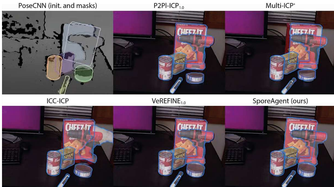
Figure 7.5: Comparison of SporeAgent with competing depth-based methods on YCB-Video. PoseCNN [8] is used as initialization and shown with the depth image.
