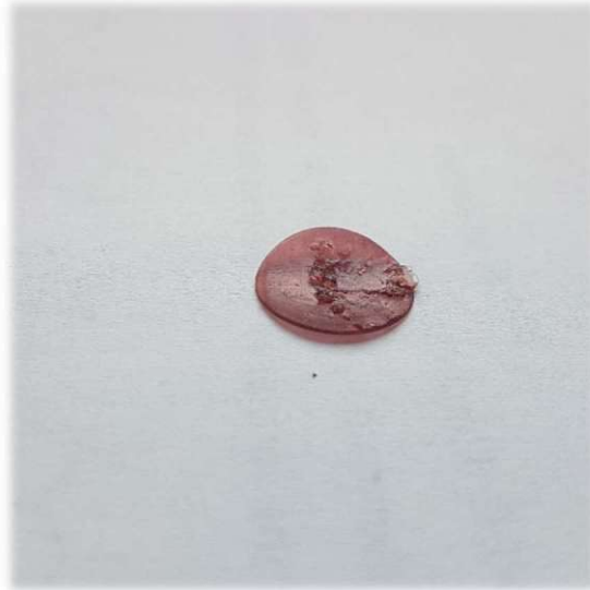
Figure 40: Printing test of the EPNovo-Formulation with TOMDA as CA at 100 °C.
