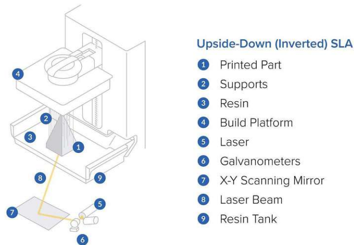
Figure 2: Schematic setup of upside-down SLA printer. [24]
