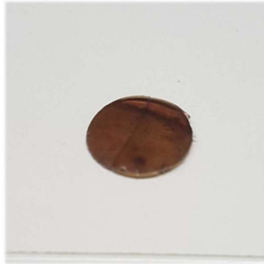
Figure 63: Printing test of PT-30 formulation at 90 °C.
