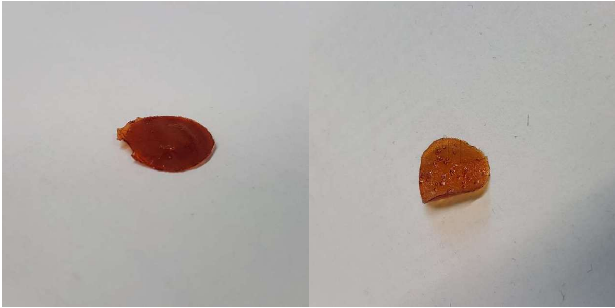
Figure 29: Printing tests (80 °C) of TOMDA (20 wt%, left) formulation and PD (40 wt%, right) formulation.
