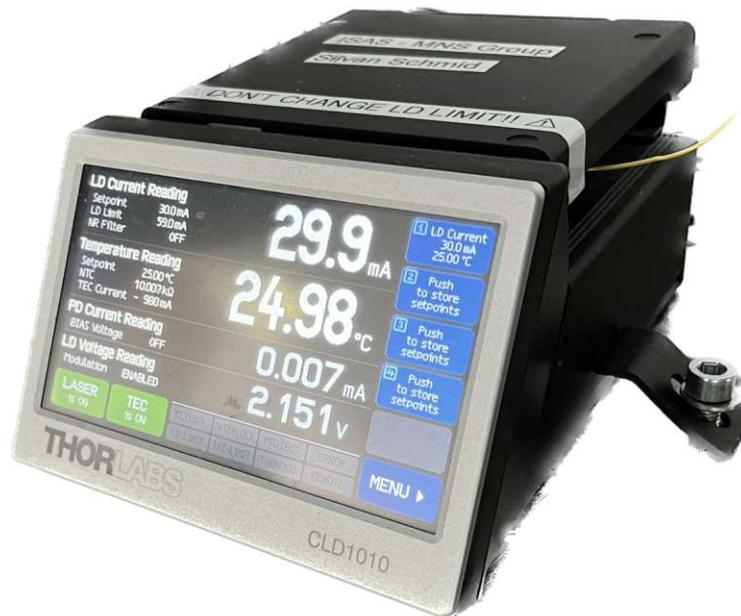
**Figure 3.6:** Laser controller: the temperature of the laser diode is kept constant at 25°C while the laser current is controlled with an external voltage signal.
