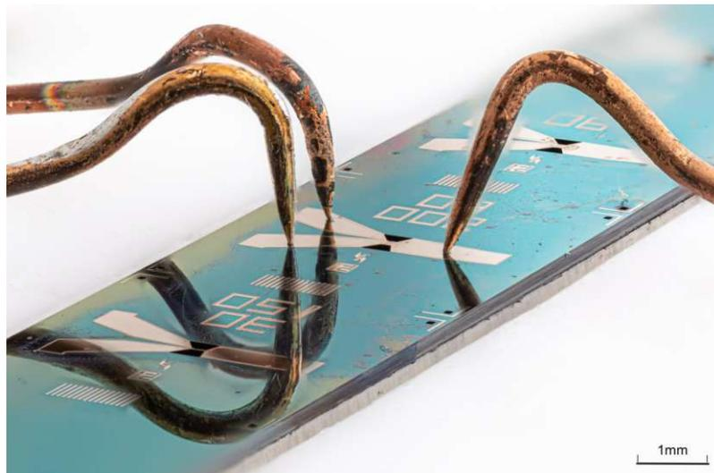
**Figure 3.26:** Close-up of a contacted device: The cantilever is being contacted with the right needle, the two needles on the left are for the big and small electrodes
