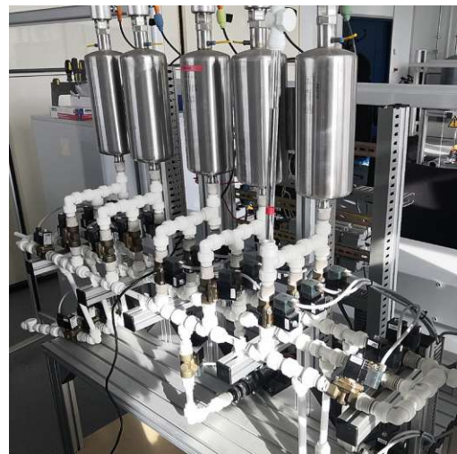
(b) Five tanks laboratory setup.
