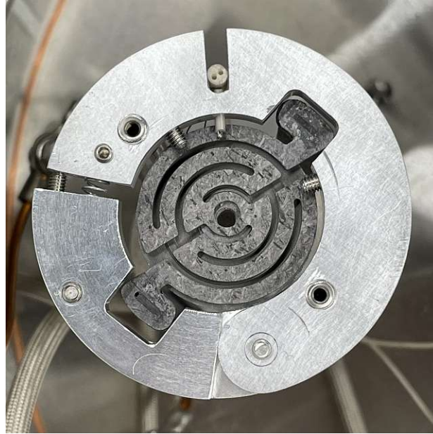
Figure 9: One version of the main sample holder, fabricated out of aluminum for easier prototyping. Cutouts for the tweezers are visible. The white pin on the top is the measurement sensor, on the left side the setscrew and the spring are visible.
