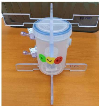
Figure 1: Set up for the irradiation under nitrogen-enriched environment.
