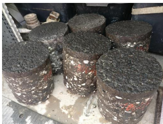
Figure 25. Obtained drill cores of the polymer-modified sample after 17 years in use.
