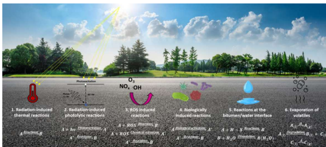
Figure 6. Illustration of possible mechanisms that lead to permanent changes in bitumen chemistry. This image was used under license from ABCDstock - stock.adobe.com.
