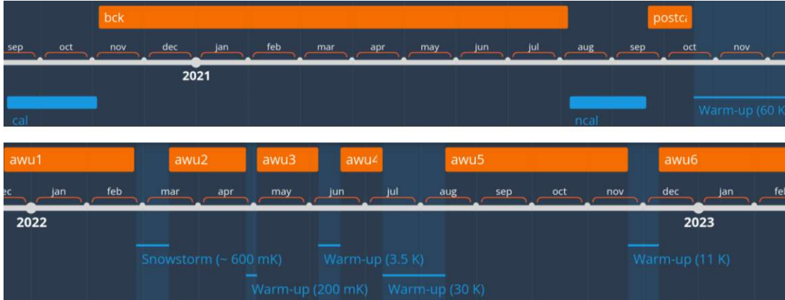
Figure 5.3: The timeline of the Run36 of CRESST-III. The data used for studying the low energy excess are drawn in orange bars, the calibration data are shown in blue bars, and the warm-ups are shown as blue lines.
