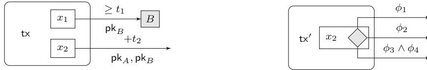
Figure F.4: (Left) Transaction \text{tx} has two outputs, one of value x_1 that can be spent by B (indicated by the gray box) with a transaction signed w.r.t. \text{pk}_B at (or after) round t_1 , and one of value x_2 that can be spent by a transaction signed w.r.t. \text{pk}_A and \text{pk}_B but only if at least t_2 rounds passed since \text{tx} was accepted on the blockchain. (Right) Transaction \text{tx}' has one input, which is the second output of \text{tx} containing x_2 coins and has only one output, which is of value x_2 and can be spent by a transaction whose witness satisfies the output condition \phi_1 \vee \phi_2 \vee (\phi_3 \wedge \phi_4) . The input of \text{tx} is not shown.
