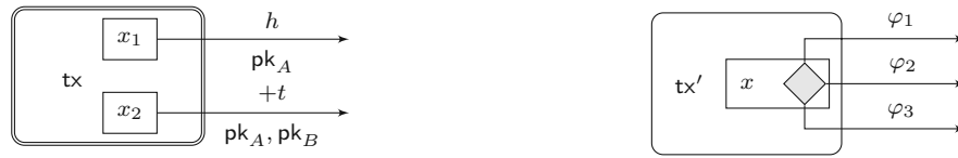
Figure 3.1: (Left) tx is published on the blockchain. The output of value x_1 can be spent by a transaction containing a preimage of h and signed w.r.t. pk_A . The output of value x_2 can be spent by a transaction signed w.r.t. pk_A and pk_B but only if at least t rounds passed since tx was accepted by the blockchain. (Right) tx' is not published yet. Its only output can be spent by a transaction whose witness satisfies \varphi_1 \vee \varphi_2 \vee \varphi_3 .
