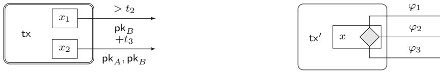
Figure 6.1: (Left) Transaction \text{tx} is published on the blockchain. The output of value x_1 can be spent by a transaction signed w.r.t. pk_B after round t_2 , and the output of value x_2 can be spent by a transaction signed w.r.t. pk_A and pk_B but only if at least t_3 rounds passed since \text{tx} was accepted by the blockchain. (Right) Transaction \text{tx}' is not published on the ledger. Its only output, which is of value x , can be spent by a transaction whose witness satisfies the output condition \varphi_1 \vee \varphi_2 \vee \varphi_3 .
