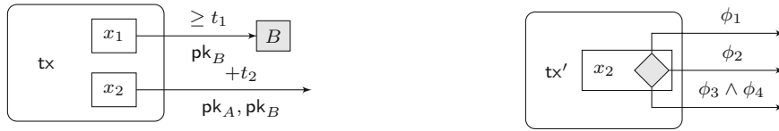
Figure 4.1: (Left) Transaction \text{tx} has two outputs, one of value x_1 that can be spent by B (indicated by the gray box) with a transaction signed w.r.t. \text{pk}_B at (or after) round t_1 , and one of value x_2 that can be spent by a transaction signed w.r.t. \text{pk}_A and \text{pk}_B but only if at least t_2 rounds passed since \text{tx} was accepted on the blockchain. (Right) Transaction \text{tx}' has one input, which is the second output of \text{tx} containing x_2 coins and has only one output, which is of value x_2 and can be spent by a transaction whose witness satisfies the output condition \phi_1 \vee \phi_2 \vee (\phi_3 \wedge \phi_4) . The input of \text{tx} is not shown.
