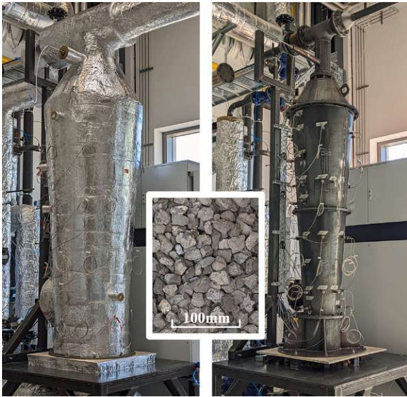
Fig. 1. PBTES test rig at the laboratory of TU Wien: with thermal insulation (left), storage material (center), without thermal insulation (right).
