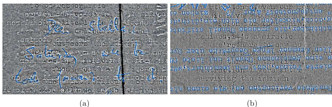
Figure 4.16: Final visualizations in the form of high-pass filtered depth maps combined with albedo maps, where inked parts of the surface appear in blue: (a) letter to Stella Musulin, (b) German typescript of ‘Joseph Weinheber’.
