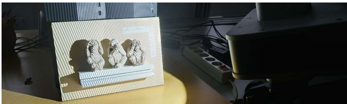
Figure 4.3: Generating ground truth for Diffuse objects dataset with a structured light scanner.
