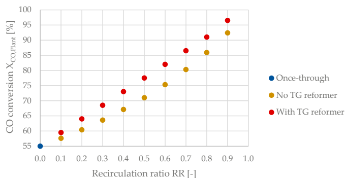
Figure 15. CO conversion at a system level as a function of the recirculation ratio.
