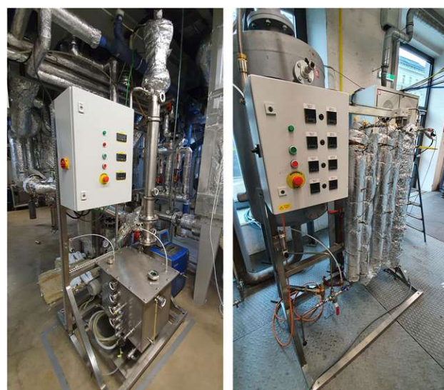
Fig. 5 Photo of the RME scrubber (left) and the activated carbon beds (right)
