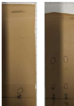
Figure S14. TLC for determining the mobile phase for the purification of THPMTGE using MPLC.
