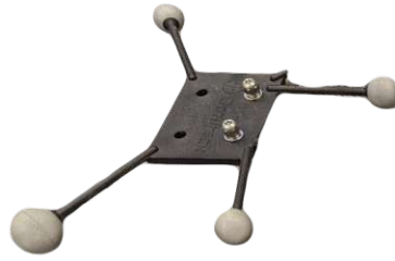
Figure 2.4: Image showing four passive markers with reflective material.
