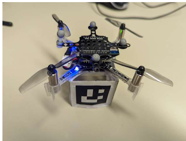
Figure 4.1: The Crazyflie UAV with attached mocap maker deck with markers.
