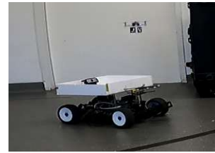
(c) Landing is initiated and the UAV lands on the platform of the moving ground vehicle.
