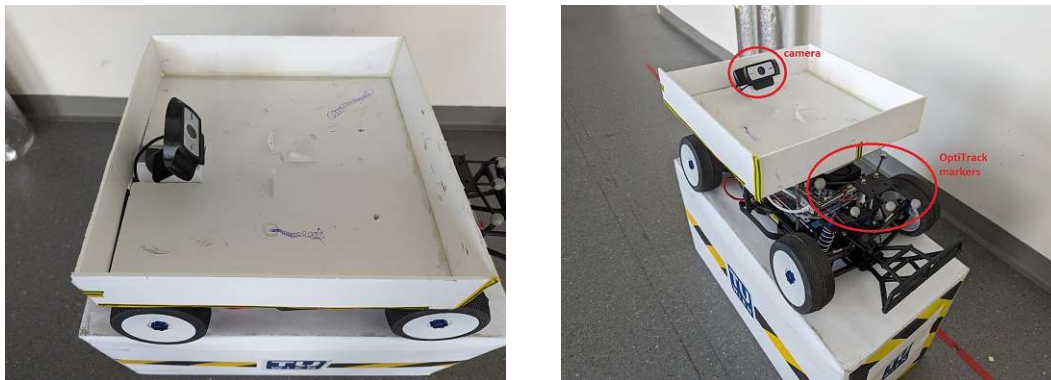
Figure 3.1: F1TENTH race care with a landing platform, OptiTrack markers, and camera.
