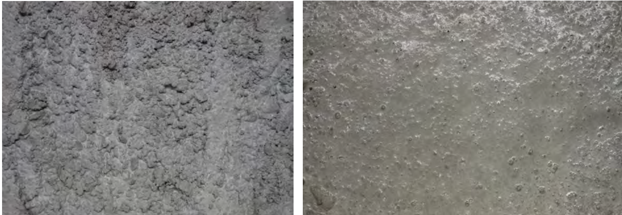
Fig. 4.18: Varying surface structure of the precast elements resulting in very different bond behavior with subsequently added in-situ concrete
