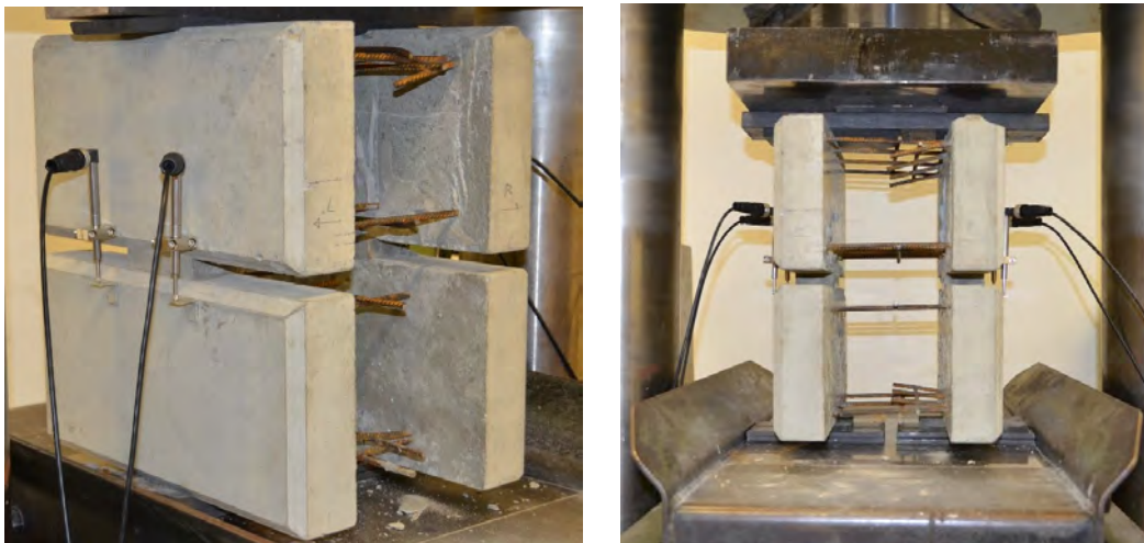
Fig. 3.6: Double wall element specimens connected by a grout joint placed in the testing machine and equipped with four linear variable differential transformers
