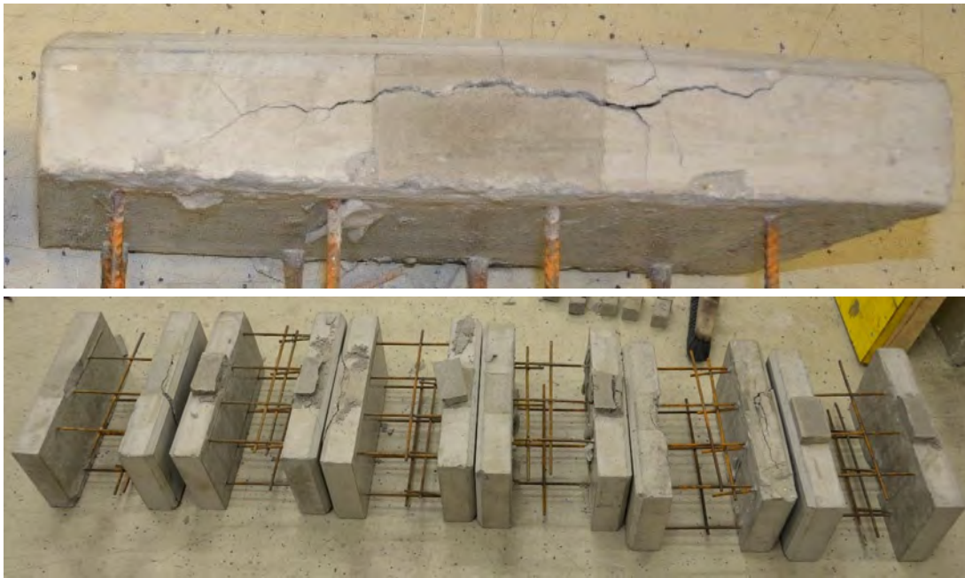
Fig. 3.7: Double wall specimens after joint compression tests using the newly designed joints
