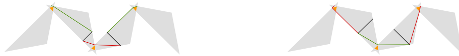
Figure 5.15: All six non-collinear triples of a fence bypassing exactly one inner polygon.
