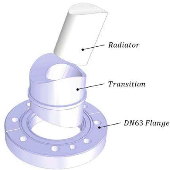
Figure 4.2: Exploding view of the radiator assembly. The design is based on a commercial DN 63 Flange, with an inner diameter of 63 mm. The cylindrical radiator is optimised for a large surface area and has a diameter of 36 mm. The radiator is coated and brazed to the transition piece.
