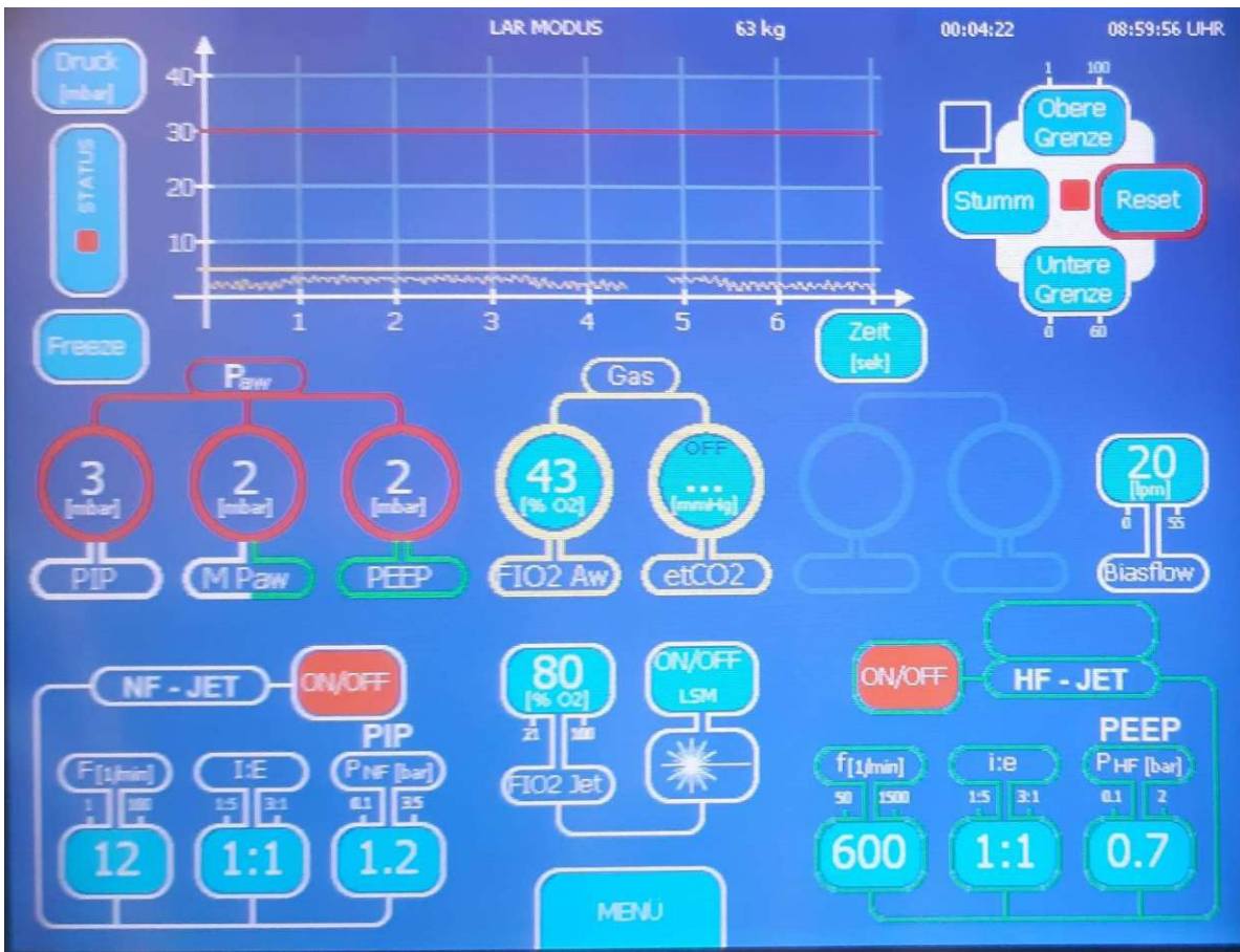
Fig 2.14 Control monitor (TwinStream™, Carl Reiner, Jet Ventilator)
