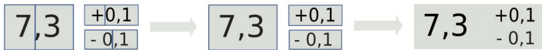
Figure 1.11: Scheibel et al. [SMRM21] use DBSCAN to merge extracted elements into complete dimension sets.
