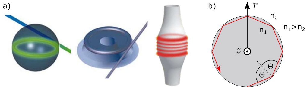
Figure 2.2: a) Different types of WGM resonators, from left to right: a microsphere, a microtoroid and a bottle microresonators. Part of the figure taken from Ref. [71]. b) Radial confinement of light in WGM resonators in a ray path picture (cross section through the equatorial plane). Light is guided along the resonator circumference via total internal reflection, which is a consequence of the relation between the refractive indices n_1 > n_2 of the surrounding vacuum ( n_2 = 1 ) and the resonator material ( n_1 > 1 ).
