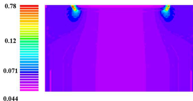
Fig. 6 2D plot of the ATP for the SPAD with a 0.5\text{-}\mu\text{m} virtual guard ring.
