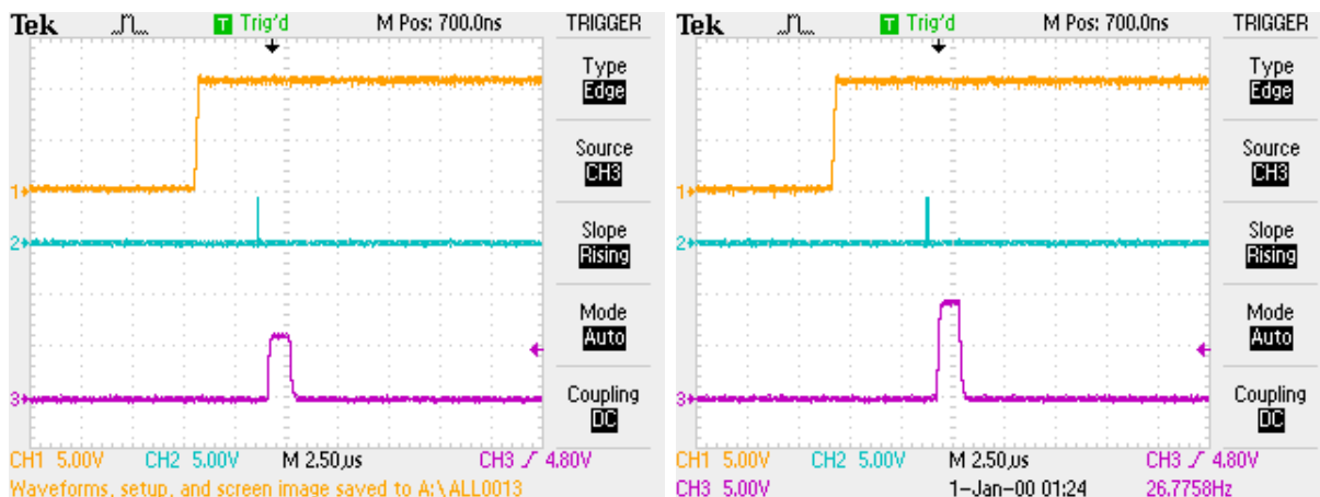
Figure 2.8.: The time difference between the function generator’s start signal (yellow) and the MCP’s stop signal (blue) determines the TAC’s output height (purple). Voltages have different offset for better visual clarity. Example signals are given for (a) short TOF and (b) long TOF.
