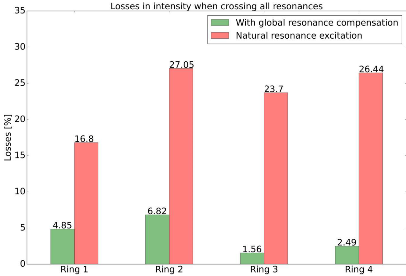
Figure 3.31: Losses crossing both normal and skew 3 rd order resonances and all normal 4 th order resonances with the global resonance compensation settings in all rings (green) and with no corrector magnets (red).
