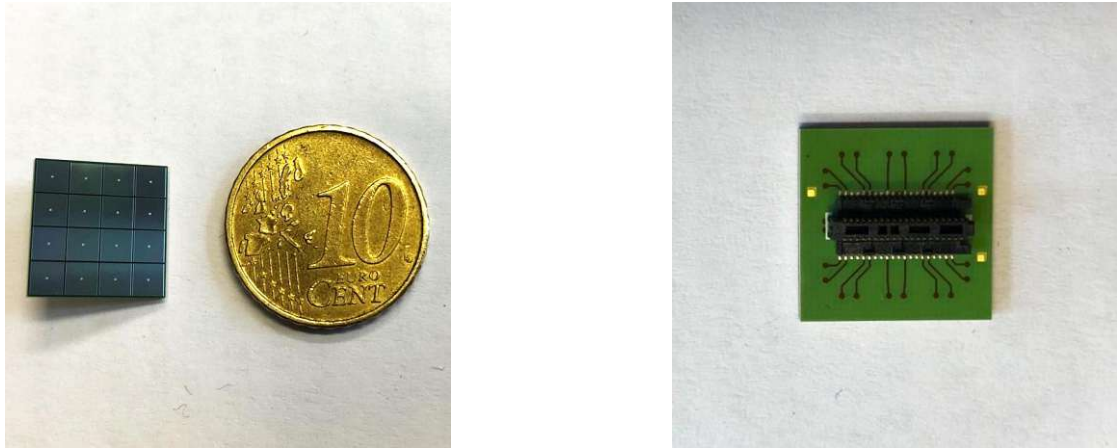
Figure 2.7.: Left: Frontside of the array with a 10-cent coin next to it for scale comparison. (SiPM: 13 mm × 13 mm, Coin: \varnothing = 19.75 mm) Right: Backside of the unit showing the connector and the anodes and cathodes of the individual SiPMs.
