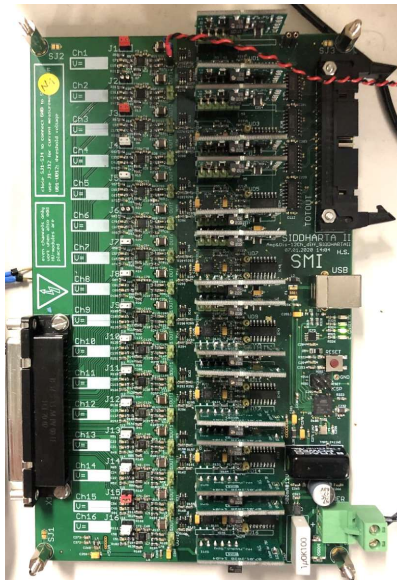
Figure 2.11.: 16 channel amplifying board produced by SMI [53]. The voltage of each channel can be set with a potentiometer individually. The board has an analogue and a TTL output and the option to be controlled remotely via USB.
