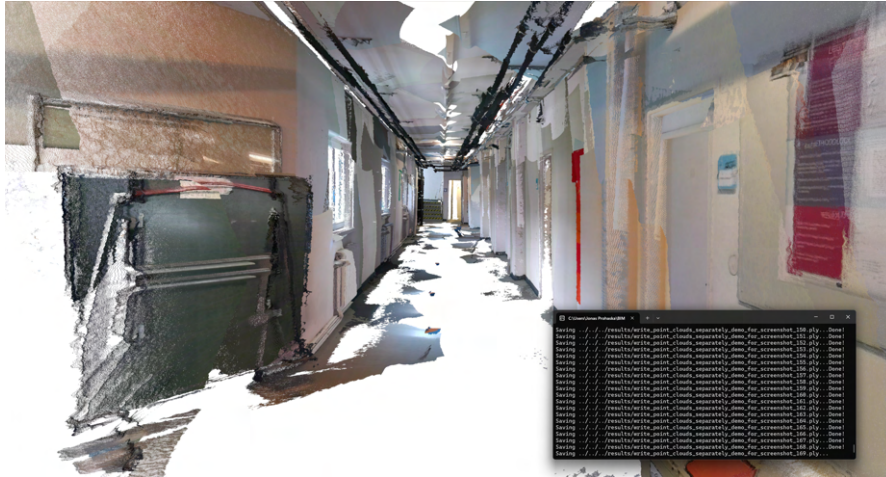
Figure 4.5: Debug visualization. Individual point clouds can be added, removed, saved or even plane segmented as one sees fit.
