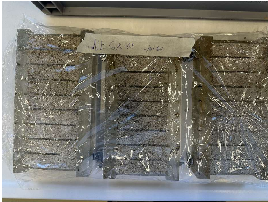
Fig. 2.8: Prisms in the 2 \times 2 \times 8 \text{ cm}^3 plexiglass molds covered with plastic foil.
