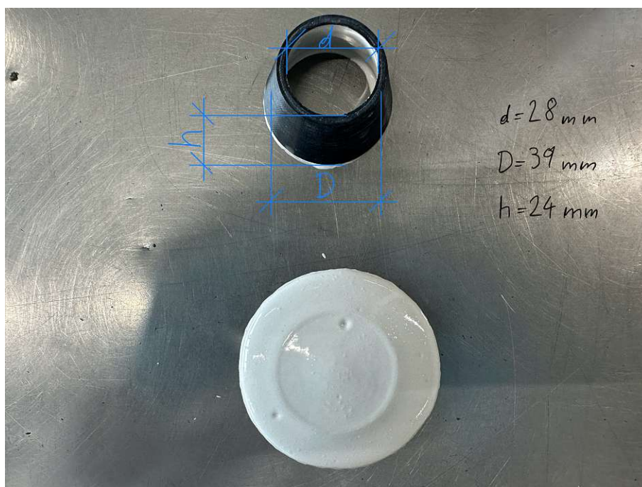
Fig. 5.1: Mini cone for the spread tests over time.
