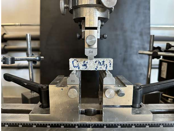
(a) 3-point bending strength test configuration.
