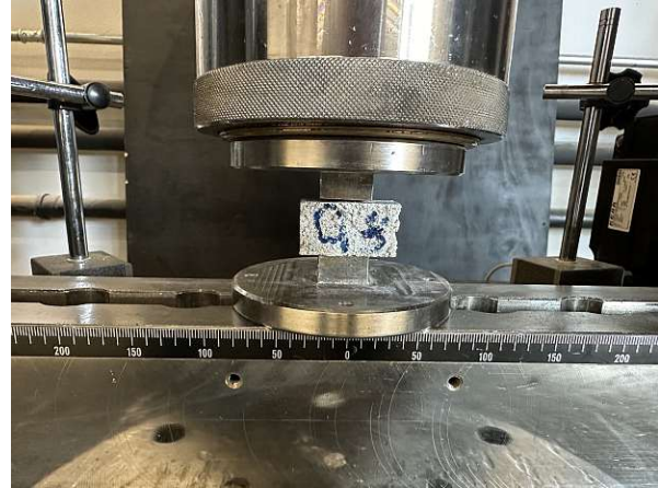
(b) Compressive strength test configuration.
