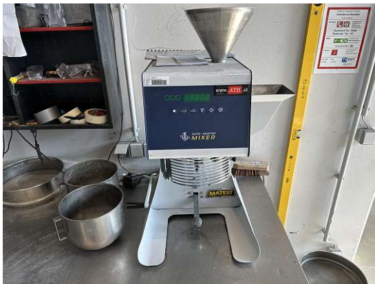
(a) Horbat mortar mixer.
