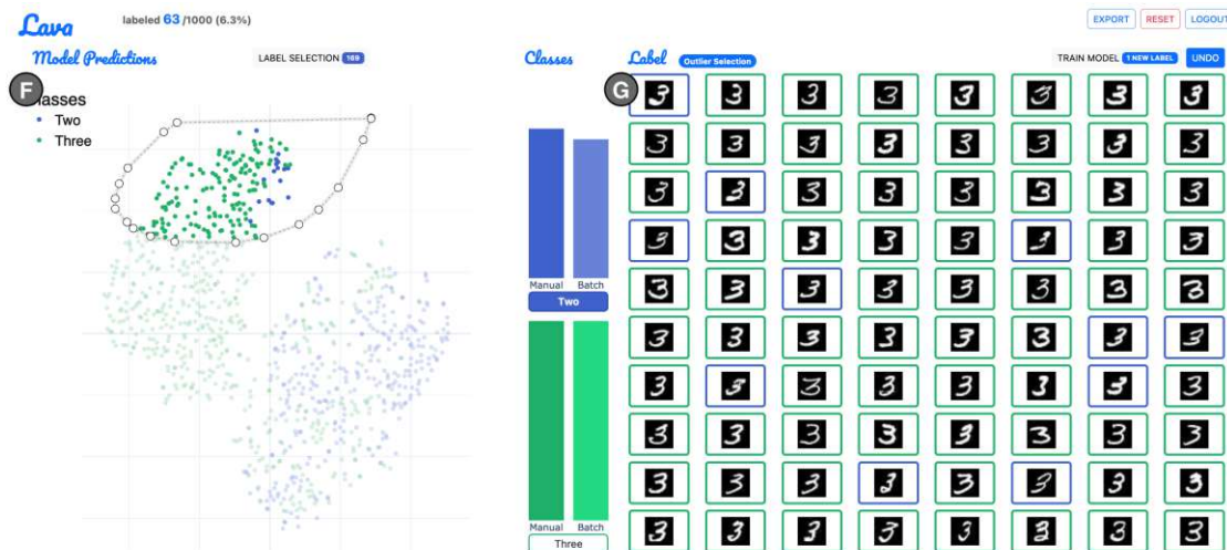
Figure 3.4: The prototype implementation of the iVIL system. The KDE plot from the cVIL prototype is replaced by a scatterplot of the t-SNE projected embeddings (F). Because the samples are not partitioned into classes, the predictions of the classification model are indicated by the border color of each image (G) in the labeling view.
