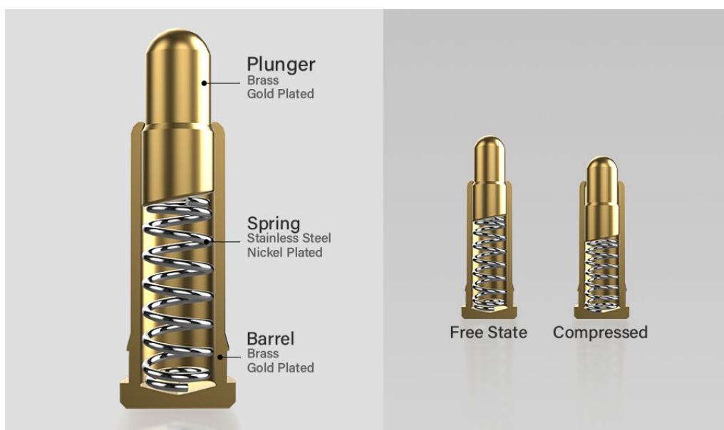
Figure 40 Spring containing pins called pogo pins, used as pins in self-fabricated chip holder [s21]
