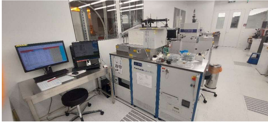
Figure 33 ZMNS RIE-ICP (PlasmalabSysem100) used for insulation layer etching
