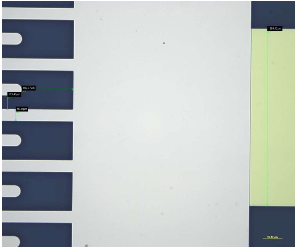
Figure 28 Post development of the second layer, a sharp border between the photoresist-covered connection line (yellow) and photoresist lacking electrodes (white) and semitransparent (glass-covered photoresist+SiN) blue background.
