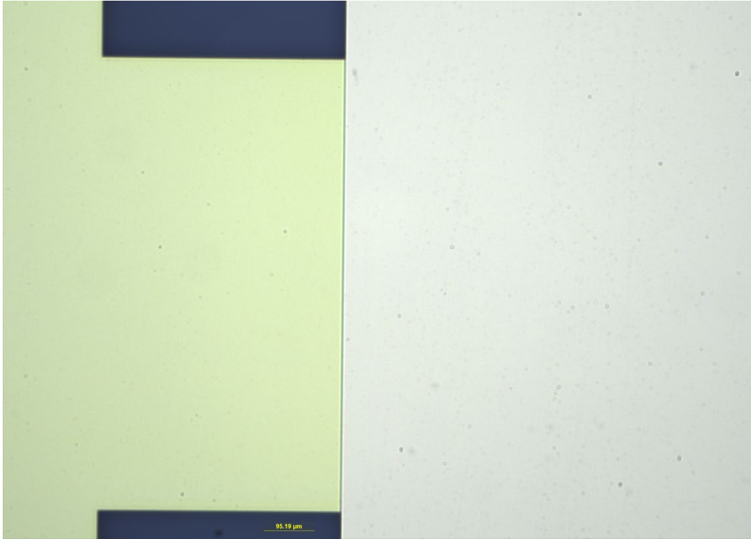
Figure 29 Post development of second layer, pads(white) without photoresist, sharp border, connection line(yellow) covered with photoresist, and semitransparent (glass-covered photoresist+SiN) blue background.
