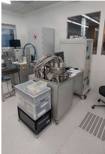
Figure 21 VonArdenne machine used for sputtering deposition (gold and titanium)
