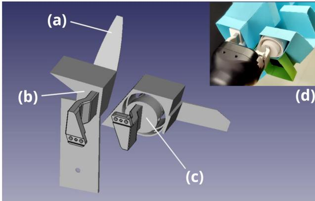
Figure 4: Gripper mounting of the Zipper Flower Tube: (a) Hook for origami, (b) gripper finger with fixed mount and downwards support plate, (c) gripper finger with rotating mount with ball bearing and side hook, (d) final assembly with paper origami mounted on the gripper.
