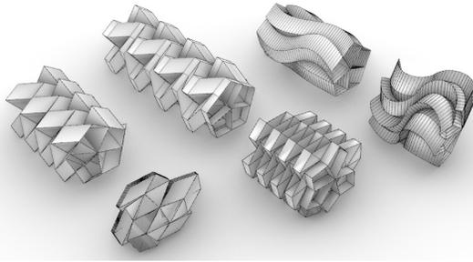
Figure 9: Zipper Flower Tubes design variations in expanded and collapsed states: (left) Flat-foldable zig-zag tube, (center) zig-up-zag-up tube with adjustable length, (right) semi-discrete flower with developable strips.
