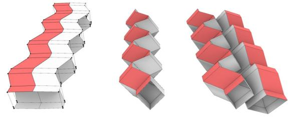
Figure 2: Zipper Flower Tube’s basis element: (Left) two flat pieces of a tubular element with connection points shown via arrows, (center) an assembled element in a half-folded state, (right) two congruent elements about to be connected via faces in a zippered fashion. By repeating the process of rotational zipper coupling, the final structure can be constructed. Note that, a row of faces in each step is marked in red as a hint to follow the orientation of the elements.
