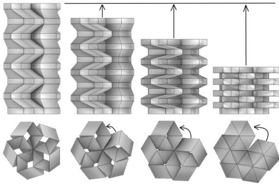
Figure 3: Expansion sequence of Zipper Flower Tube in four steps from right to left. Arrows illustrate the direction of the expansion in the top view (top), and the rotation of the cross sections in the front view (bottom). By fixing the positions of the tubes, additional resistance can be obtained.
