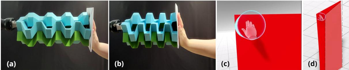
Figure 1: Stiffness simulation with our Zipper Flower Tube: (a) User's hand encounters uncompressed Origami, (b) hand presses against Origami, (c) user's view in VR while pressing against a virtual wall, and (d) side view on the virtual wall deformed from its normal state (shown in semi-transparent grey).
