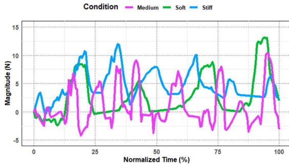
Figure 6: Typical temporal evolution of the magnitude of the gripper sensor data over time per condition (soft in green, medium in purple, and stiff in blue).
