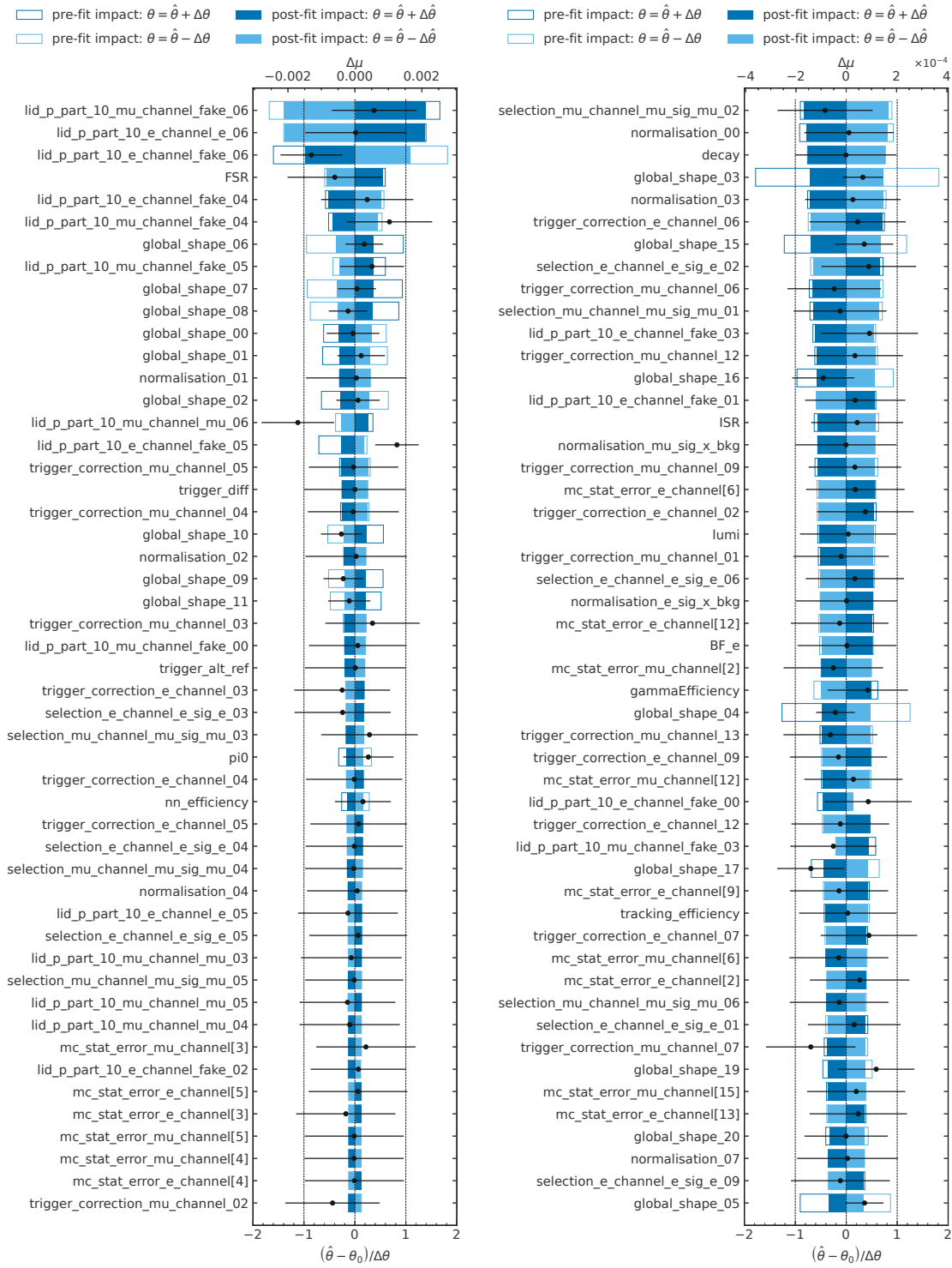
Figure 4.59: Ranking plot showing the impact of varying the different nuisance parameters within their associate uncertainties on R_\mu . For the pre-fit impact \Delta\theta denotes the uncertainty provided in the constraint term of the nuisance parameter, while for the post-fit impact, \Delta\hat{\theta} is the uncertainty as obtained from the fit. In addition, the pull values and associated uncertainties of the nuisance parameters are overlaid with black markers.
