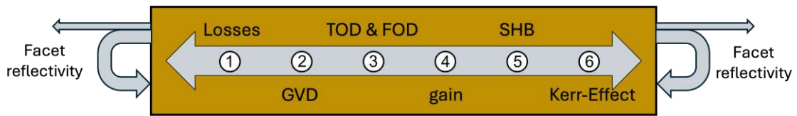
Figure 2.4: Schematic drawing of a Fabry-Pérot laser cavity outlining the main components of the analytical description: losses, group velocity dispersion (GVD), third and fourth-order group velocity dispersion (TOD and FOD), gain, spatial hole burning (SHB), and the Kerr-effect.
