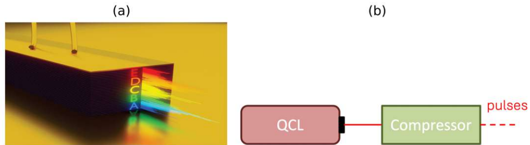
Figure 1.2: Broadband sources for spectroscopic applications: (a) heterogeneous QCL, (b) short pulses generated by the combination of a QCL emitting an optical frequency comb with an optical compressor, potentially triggering non-linear optical effects to broaden the spectrum. Source for (a): [20]
