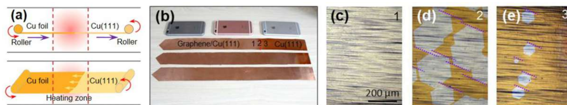
Figure 1.4: Figure to illustrate highly scalable production of large-scale single-crystal monolayer graphene on copper via CVD. (a) Schematic of experimental design for the continuous production of single-crystal Cu(111) foil with a hot temperature zone at the center of the furnace tube. (b) Cu(111) foils with graphene coverages of ~60 % (top), ~90 % (middle) and 100 % (bottom). (c-e) Optical images representative of regions marked in (b) with 1-3 respectively showing areas (c) fully covered by graphene, (d) covered by large aligned graphene islands and (e) covered by small aligned graphene islands. (Adapted from Xu et al. 30 )
