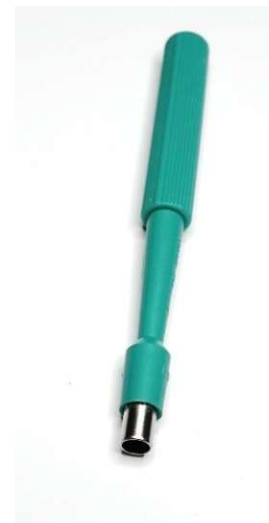
Figure 21. Picture of the biopsy punch used to cut small discs out of the wing. © Alexander M. Bürger
