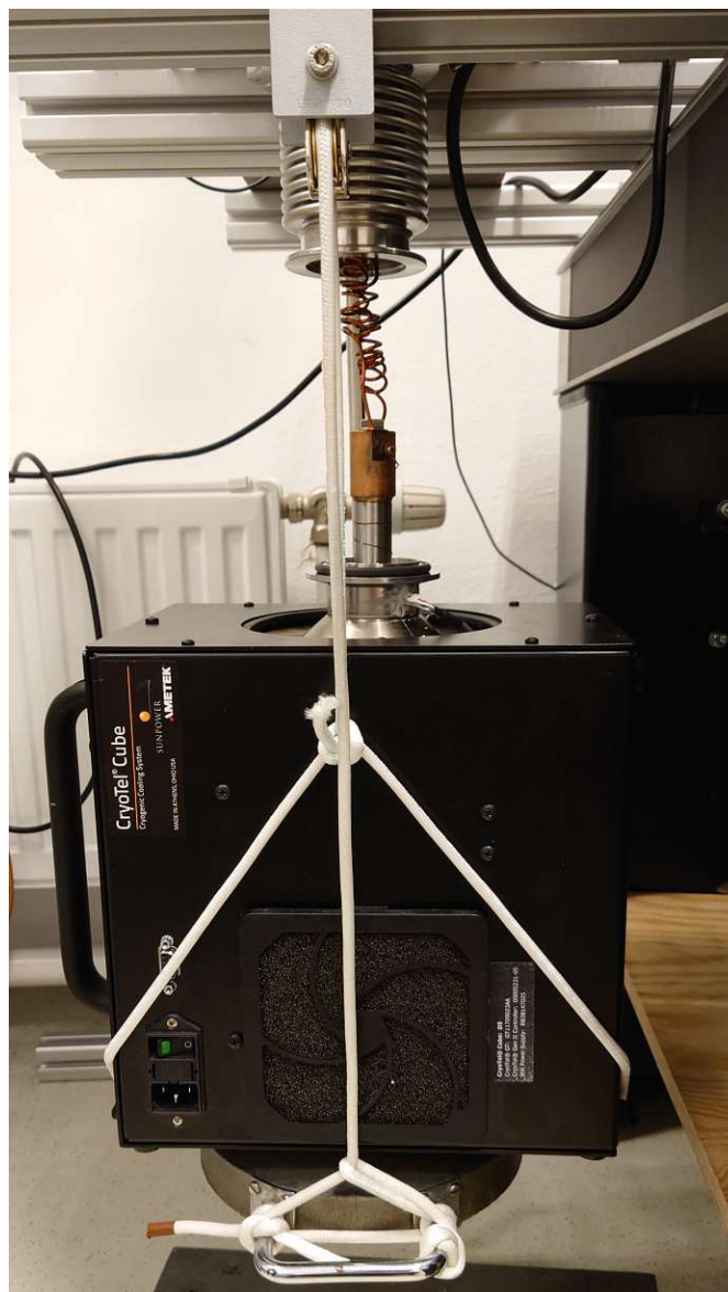
FIGURE 5.4: Sunpower cryocube suspended with rope and a piece of lead of the same weight as the cube. This contraption was needed to avoid pressure on the vacuum connection on the cube, as it was too weak to resist any stress. The whole suspension and bellows system was designed such that it could be moved, as the holder needed to be able to move up and down for transmission measurements. The copper wires that are meant to cool the holder were shaped into a spring to provide some longitudinal motion freedom.
