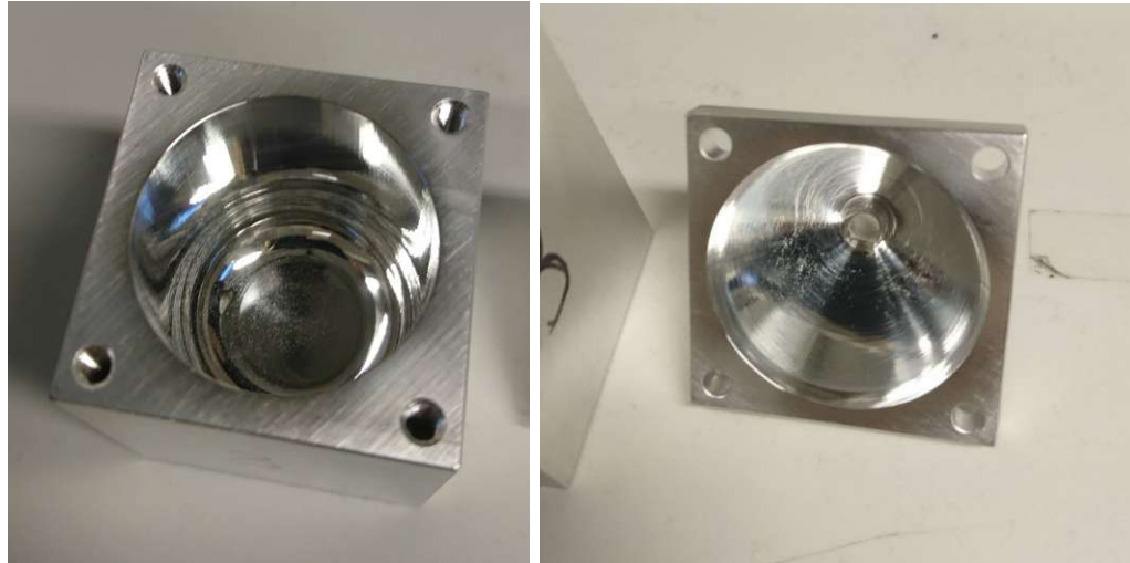
FIGURE 3.9: Aluminum container for ^{229}\text{Th} powder and funnel that can be mounted on top of the container. The insides of both components was polished to optical quality using diamond paste to reduce powder sticking to the walls. One milligram of powder can be barely seen on the bottom of the container.
