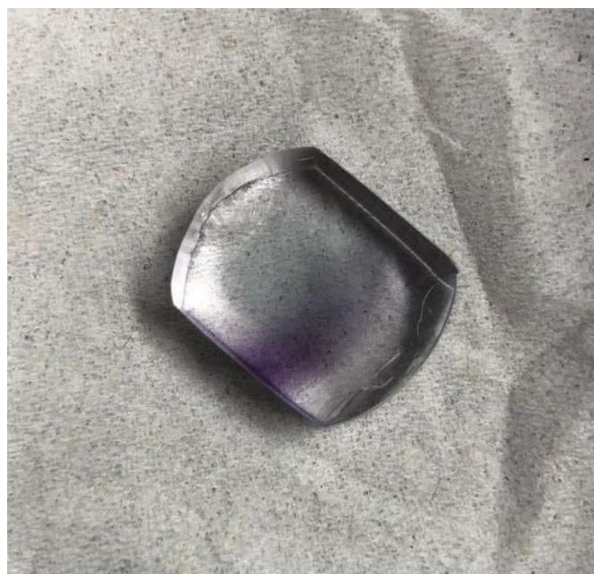
FIGURE 4.55: ^{229}\text{Th}:\text{CaF}_2 crystal V057 after fluoride annealing (no glitter observable) and subsequent damaging using a krypton excimer lamp for 24 hrs. The glitter must have prevented this type of damage by restricting motion of fluorides because this was not observed in the experiments in section 5.6.1. Annealing to 550 °C removed the visible damage but never the glitter.
