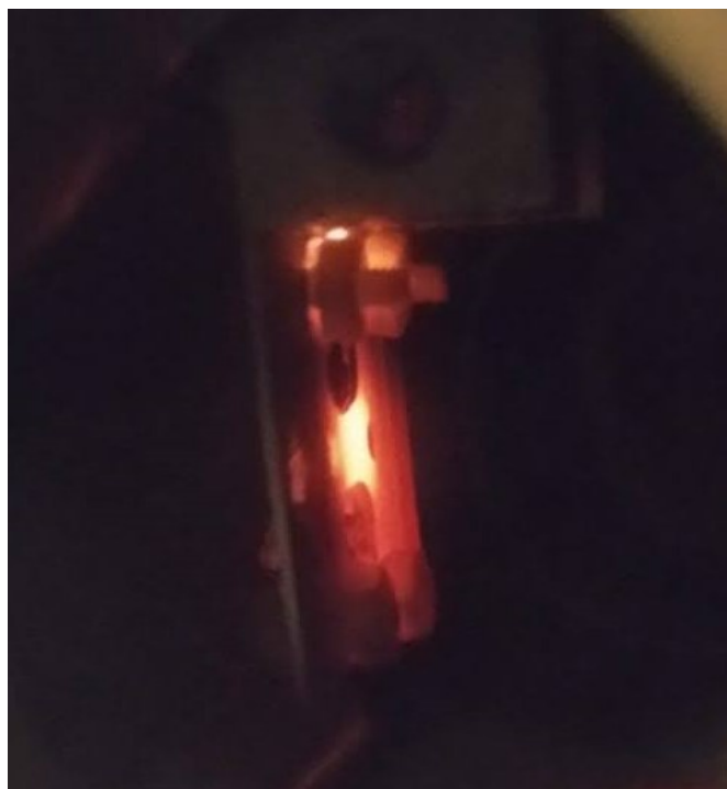
FIGURE 4.33: Zoom through a vacuum viewport of the annealing holder while in operation. Temperatures above 800^\circ\text{C} were reached to create this glow.
