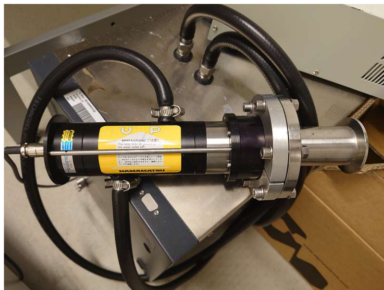
FIGURE 4.7: \text{D}_2 arc discharge Hamamatsu L1835 lamp. Connector to KF40 vacuum connection is shown together with water cooling tubes.
