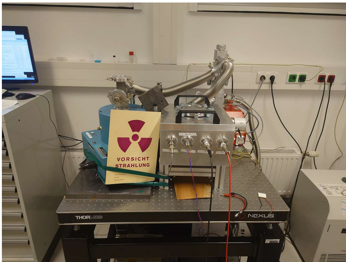
FIGURE 4.41: Long integration setup in the lab, as in 4.39. Note the lead shielding between crystal and detector. This was needed due to the high activities produced through neutron irradiation of \text{CaF}_2 crystals.
