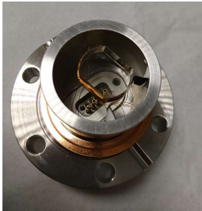
FIGURE 4.44: Simple ohmic heating holder. The V057 ^{229}\text{Th}:\text{CaF}_2 crystal was wrapped in a kapton isolated copper wire effectively producing a coil. The coil, a temperature sensor and holding mechanism were secured using torrseal. Using a vacuum electrical feedthrough and a 12V power supply the crystal was heated. The crystal was put in front of a McPherson 234/302 spectrometer with a camera at the end to measure the temperature dependent radioluminescence.
