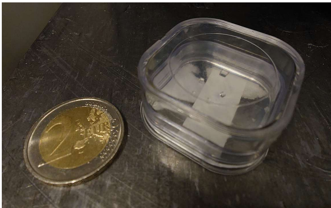
FIGURE 3.18: Four 1\text{ mm}^3 and one 4\text{ mm}^3 ^{229}\text{Th}:\text{CaF}_2 crystals cut and polished using above techniques.
