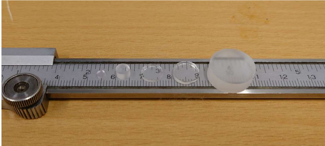
FIGURE 3.7: The experimental steps undertaken reducing the crystal diameter from 17 mm to 3.2 mm. Crystals were cut to different lengths. Diameters were limited by the diameters available for seed crystals: 17 mm, 10 mm, 8 mm and 5 mm. The last miniaturization step to 3.2 mm was done by milling down a 5 mm diameter seed by an optics company (Hyperion optics).
