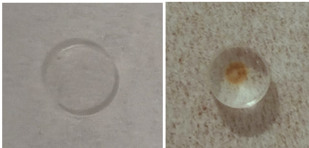
FIGURE 5.14: Crystal before and after damaging by VUV irradiation. An orange color is produced which is possibly due to F, M or N centers or due to deposition of cracked hydrocarbons that are leftover in the vacuum system.
