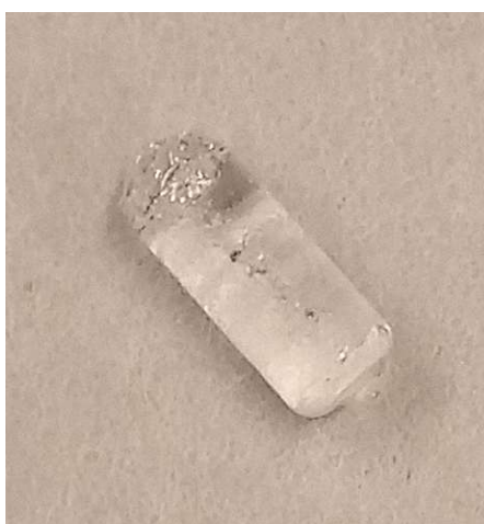
FIGURE 3.20: \text{CaF}_2 crystal grown with a vortex of bubbles. The origin of these vortices is unknown, but radial/longitudinal temperature fluctuations and convection could be a cause. Often more and stronger vortices were seen for crystals that were grown at very high temperatures, increasing boiling.
