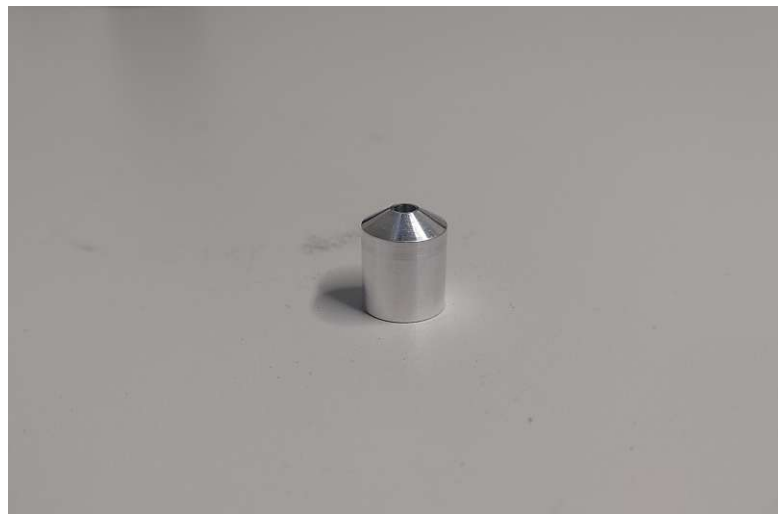
FIGURE 3.10: Small funnel used to fill the small seed crystal (see figure 3.6). This funnel connects to the crystal and the large funnel such that powder can be filled from the large container up to the crystal with minimal losses.
