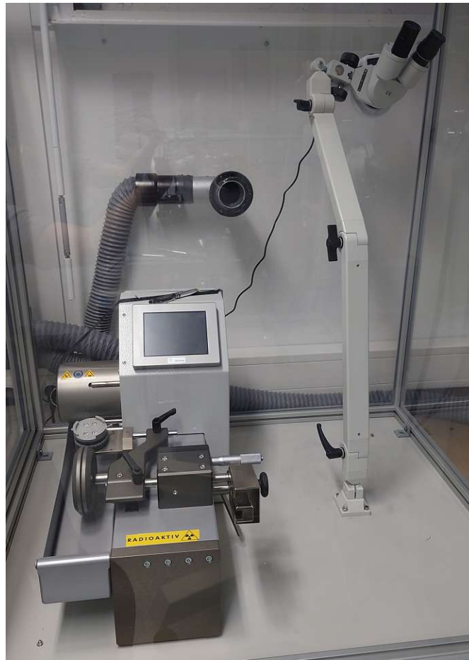
FIGURE 3.16: Diamondtec wiresaw used to cut the small crystals. The diamond wire had a diameter of 0.08 mm. By using a rotation stage the crystals could be accurately cut.
