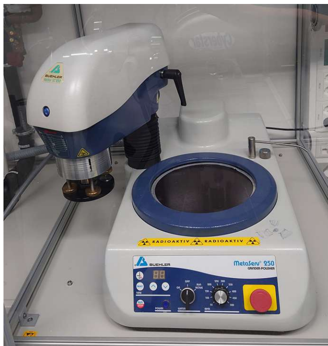
FIGURE 3.17: Buehler polisher used to polish the crystals. Since the holders were not suited for the small crystals often polishing was done by hand. A P4000 SiC polishing paper was used to polish the cut crystal surfaces.
