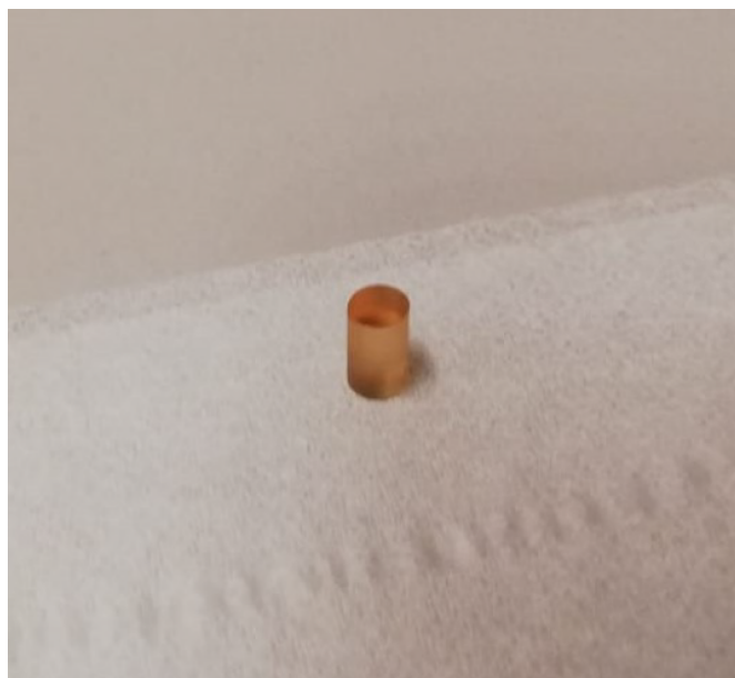
FIGURE 6.14: Undoped \text{CaF}_2 crystal that was irradiated by neutrons in the TRIGA mark II reactor for 3 hours. The orange coloring is indicative of many highly localized defect centers in the form of F, M and N centers. Any larger agglomerations of defects would color the crystals purple as is seen in heavily damaged \text{CaF}_2 with higher concentrations of F centers [111]. This indicates this crystal has a low F center concentration which are not agglomerated.
