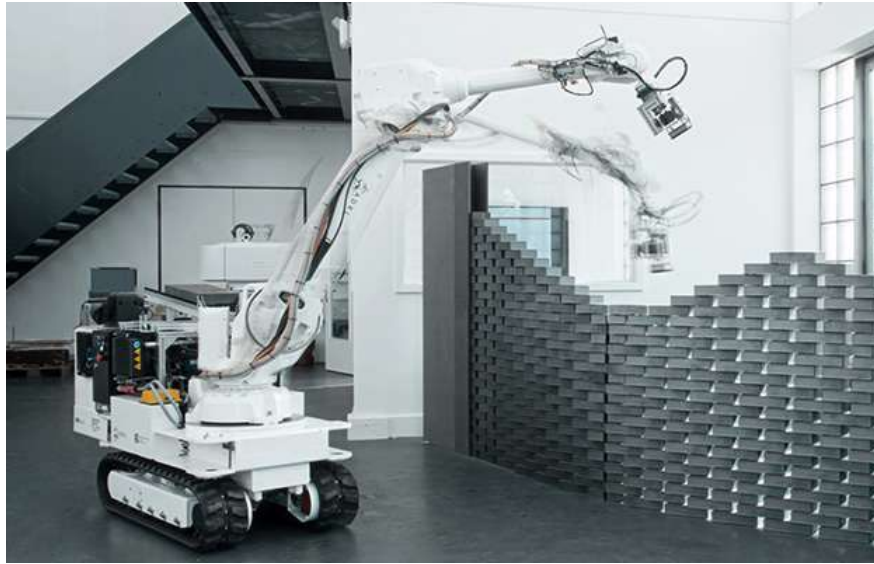
Figure 2.17: In-Situ Fabricator, Gifthaler, Sandy, Dörfler et al., 2015.
