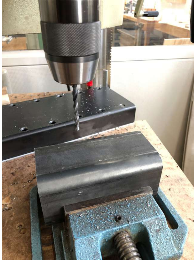
Drilling holes into the connecting pieces.
