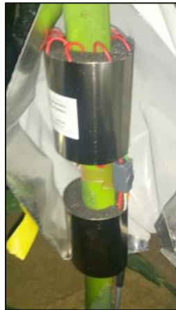
Figure 2.2: Example of sap flow system EMS 62. The thermocouples are inserted 15cm apart, with the heating elements installed at the upper section.
