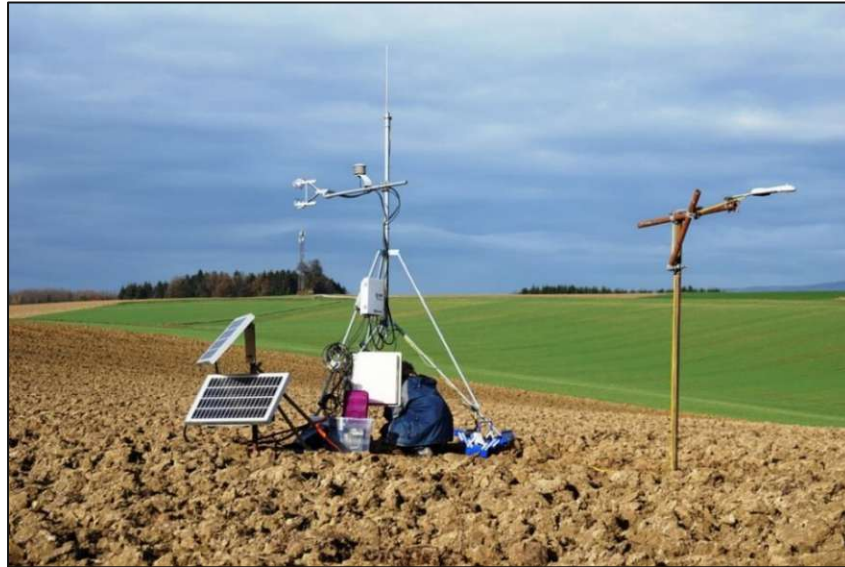
Figure 4.3: Eddy covariance system (IRGASON) mounted on a 2.5 m tripod at a mobile station.
