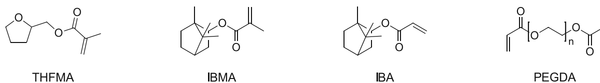
Figure 33: Reactive diluents for vat photopolymerization of vegetable oils. Tetrahydrofurfuryl methacrylate (THFMA), isobornyl methacrylate (IBMA), isobornyl acrylate (IBA) and poly(ethylene glycol) diacrylate (PEGDA).
