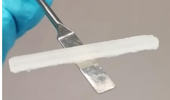
Figure 112: DMTA specimen of poly(IPN30PHTE).
